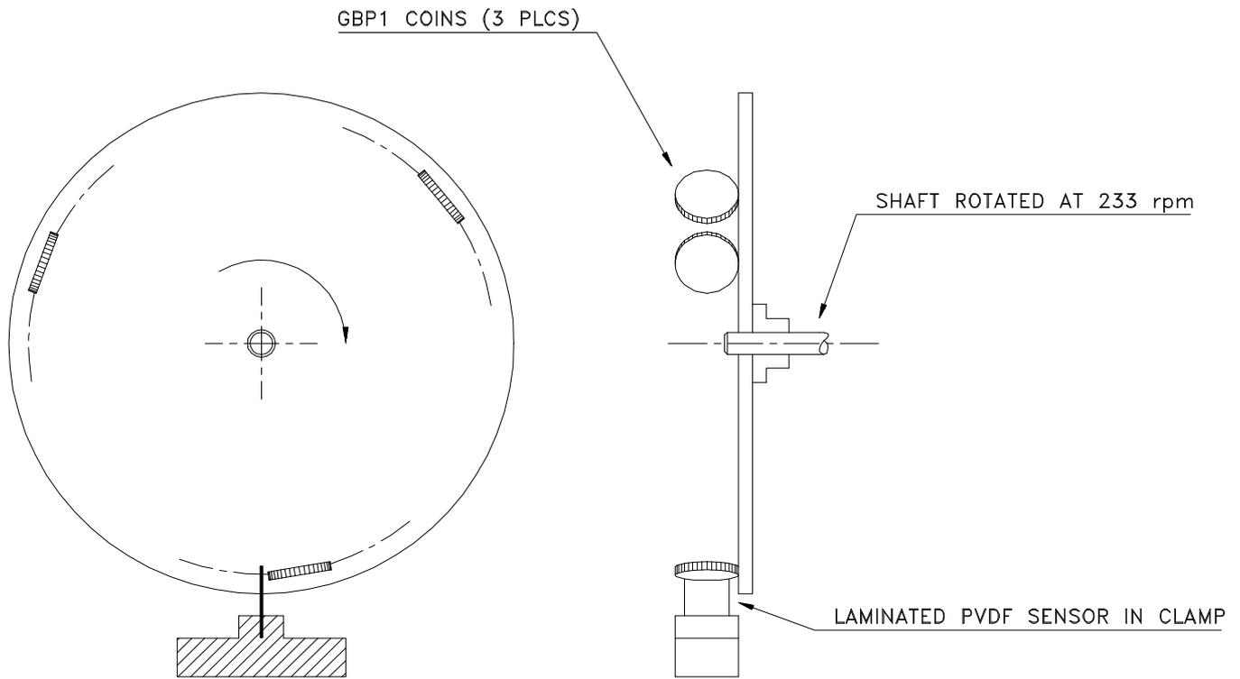
COIN SENSOR ENDURANCE TEST SET-UP
